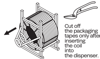
Install the coil in the dispenser IN THE DIRECTION of the arrow. The direction of unwinding is the same as the direction of the arrow.
