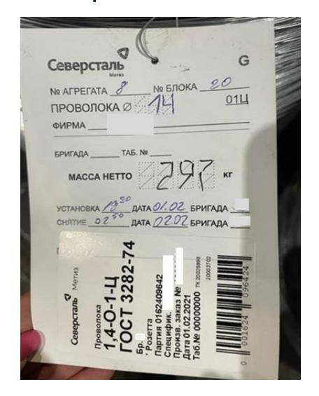
Annex: an identification tag containing a barcode, production line/drawing machine number (fixed on the product itself).
