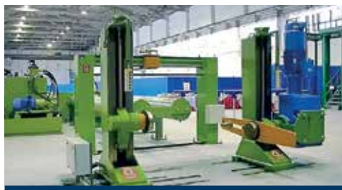
Static stretching for big diameters Ø 19-90 mm
