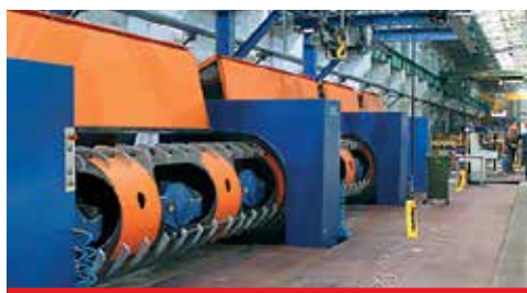
Dynamic stretching for mid-diameters Ø 15-35 mm
