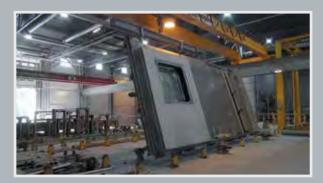
Production of "sandwich panel" using fiber concrete together with Lipabetoni. Pieksämäki, Finland.
