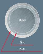
For applying ZnAl coating, Zinc coating is applied first. Wire section has two layers of coating (Zn and ZnAI) due to the different temperatures of application.
